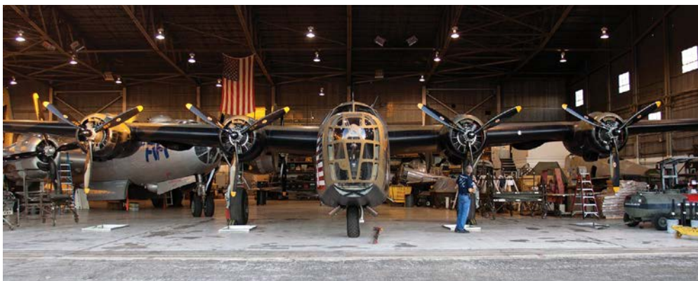
Diamond Lil is powered by four Pratt & Whitney R-1830 Twin Wasp engines.
