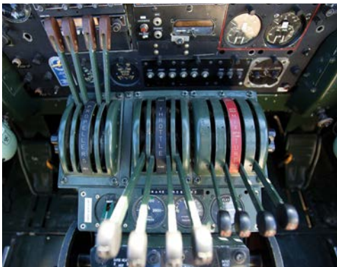
The power quadrant bristles with levers.
