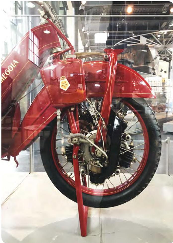
An early 20th century German Megola motorcycle powered by a wheel-mounted rotary engine.
